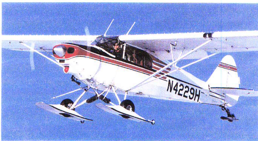
The main wheels extend only 1.5 inches below the ski bottom.
