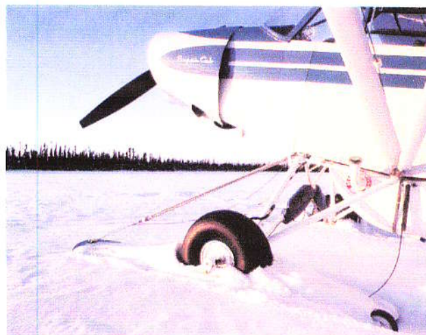
Second generation LW2500 skis. Note the position of the rear wheel.
